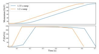
Figure 3: The 1.2 s ramp vs. the 1.33 s Main injector ramp. The rate of change of momentum  $\dot{P}$  is also shown.
