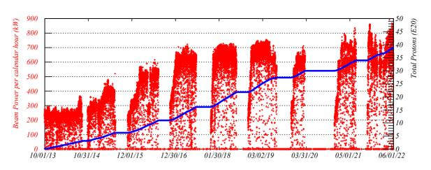
Figure 2: The hourly beam power to NuMI and the total protons delivered since the end of the long shutdown in 2013.
