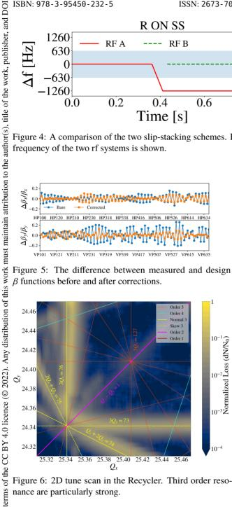
Figure 6: 2D tune scan in the Recycler. Third order resonance are particularly strong.
