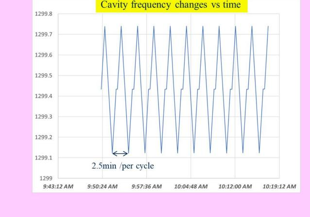
At VTS three cool-down warm up cycles: (1) 130 + (2) 270 + (3) 640 = 1040 cycles
