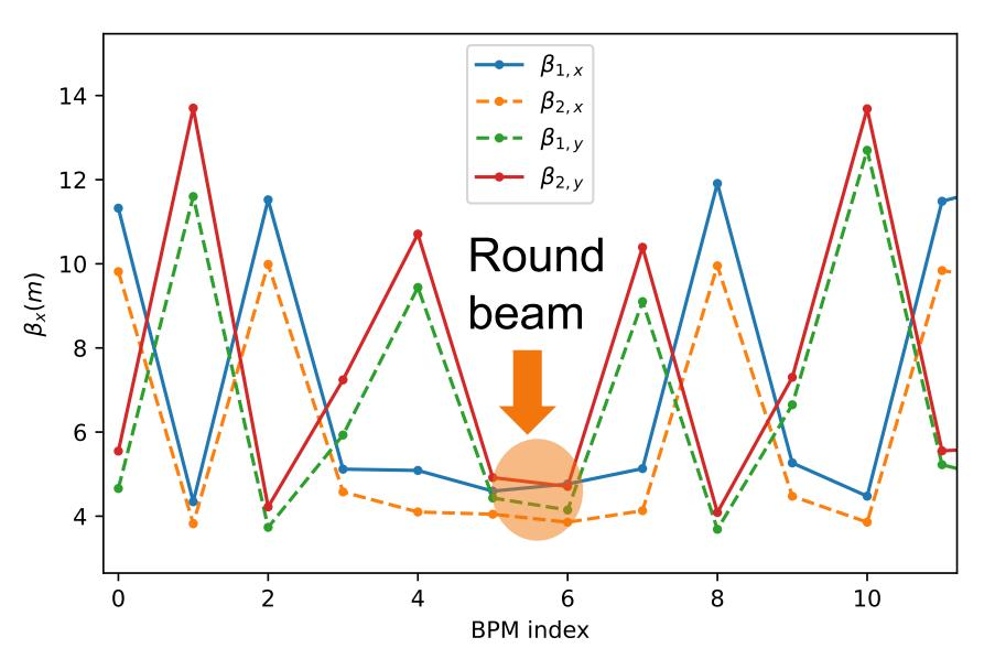
Measured coupled Twiss for one supercell
