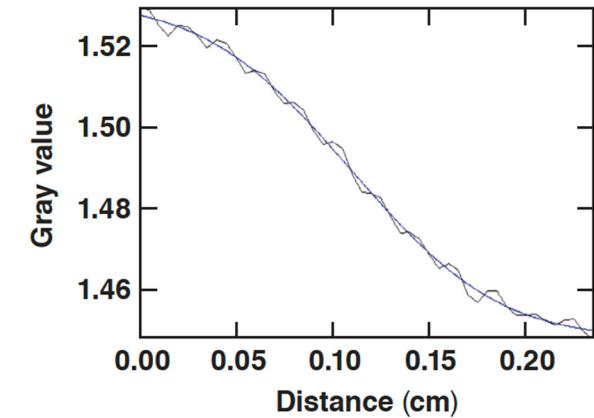
Resolution measurement on tungsten radiography object
