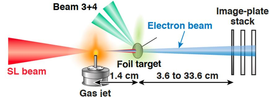
Schematic of eRad of driven CH foil
