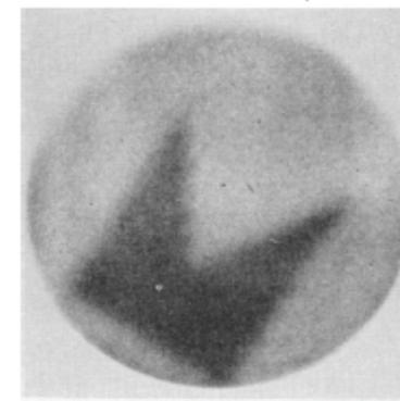
Fig. 1. Proton radiograph of aluminum absorber 7 cm in diameter and  $18 \text{ g/cm}^2$  thick, with an additional thickness of  $0.035\text{-g/cm}^2$  aluminum foil, cut in the shape of a pennant, inserted at a depth of  $9 \text{ g/cm}^2$ . The addition of 0.2 percent to the total thickness produces a substantially darker area on the film.
