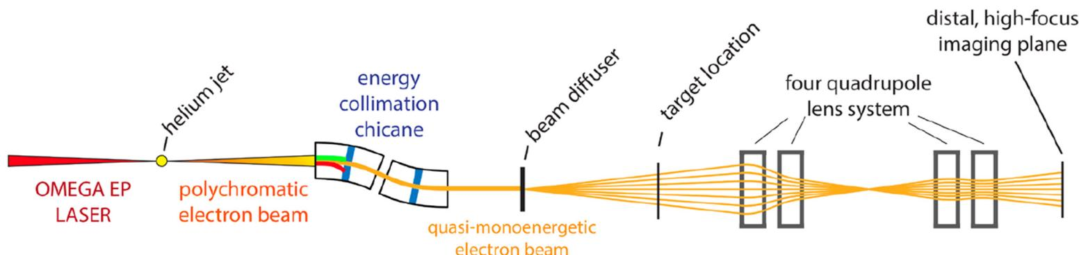
Chicane and magnetic optic design for OMEGA-EP
