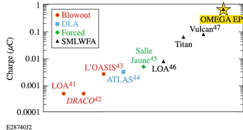
Comparison of laser driver vs electron beam bunch charge\*
