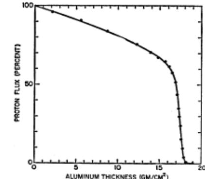
Fig. 2. Proton flux as a function of depth in aluminum. The steeply falling portion of the curve near  $18 \text{ g/cm}^2$  is used to obtain the high contrast of Fig. 1.
