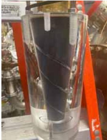
Custom designed HV plug with cooling channel
