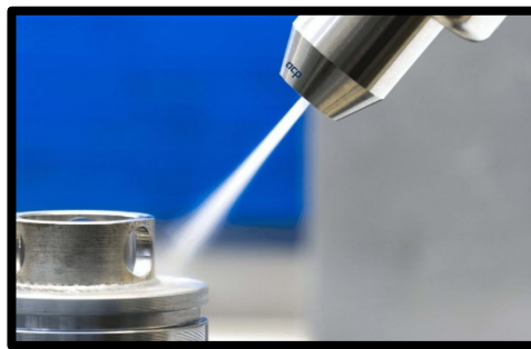
CO2 Snow-jet cleaning
