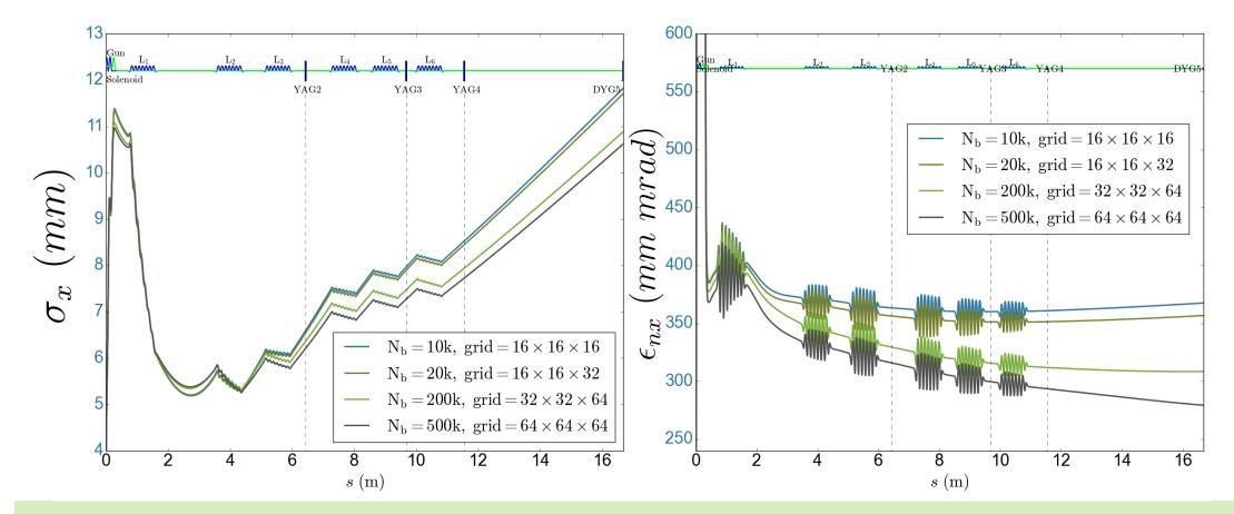
In case where the beam charge is very large more convergence check with **increased number of particles in each cell** is needed
