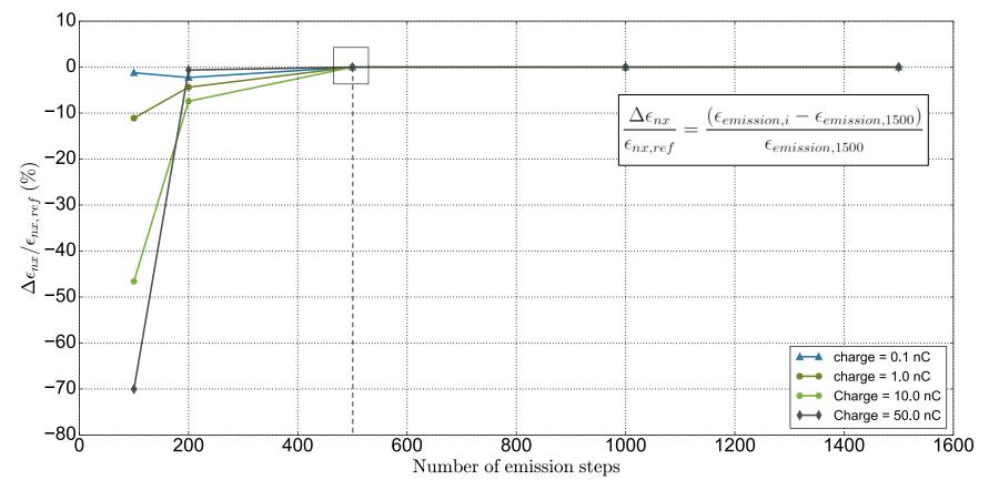
Emittance difference is minimized and converged when the emission step becomes 500 or larger
