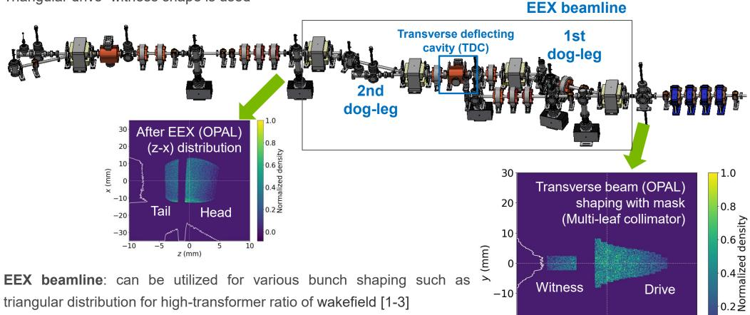
Please see N. Majernik et. al., TUPA85 paper for more details on EEX-based longitudinal bunch shaping using <u>multi-leaf collimator</u>
