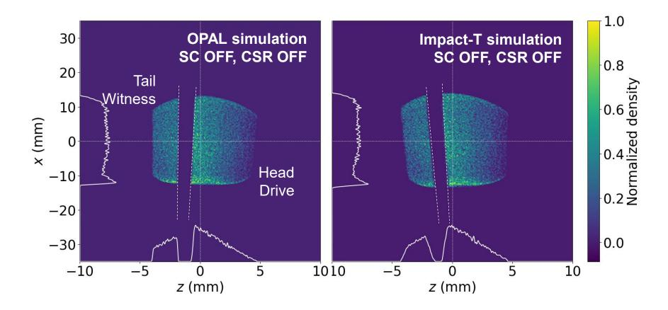
Without any collective effects is distortion is expected to be due to slightly different TDC phase setting
