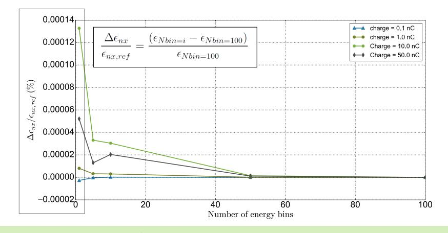
Difference is very small we do not need to consider using many number of energy bins for high-resolution for space charge with different fractional energy distribution along the bunch
