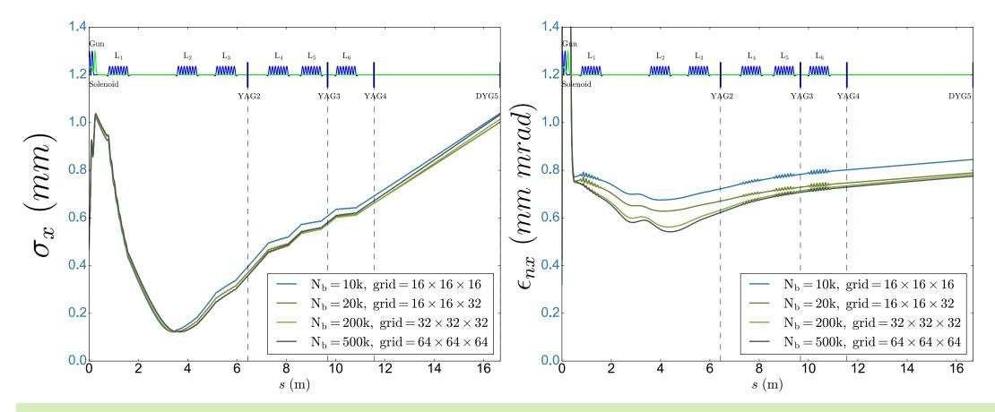
For parameter scan purpose to check the trend  $\longrightarrow$  10k particles and small grid points are enough For precise value from the simulation  $\implies$  200k particles with increased grid points are required
