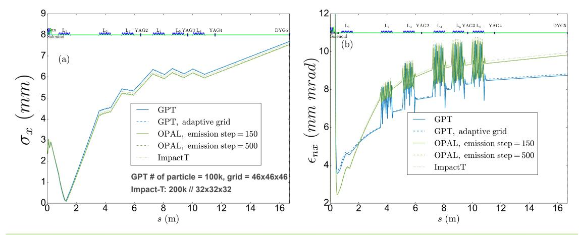
By using larger UV radius **Mitigation of space charge force** near cathode Simulation results are reasonably agreed in terms of trend (except for the emittance after RF gun)
